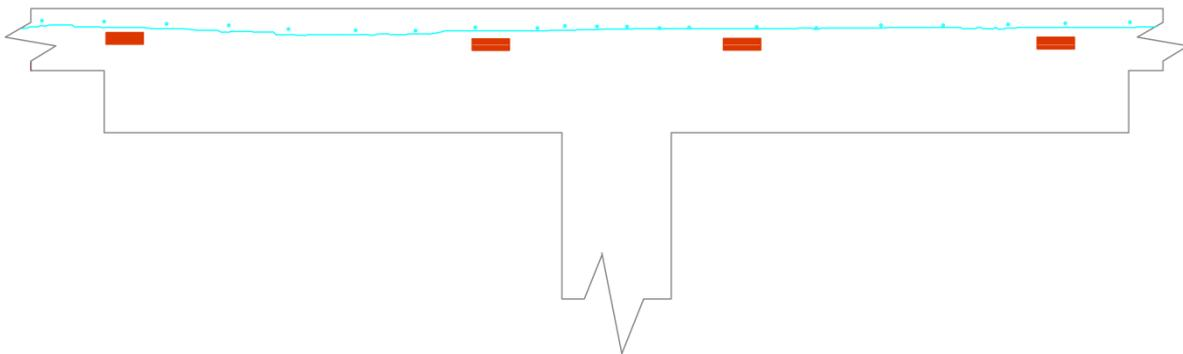
**Figure 4: Cross Section through the slab and dropdown panel, showing position of PT Ducts and reinforcement**
