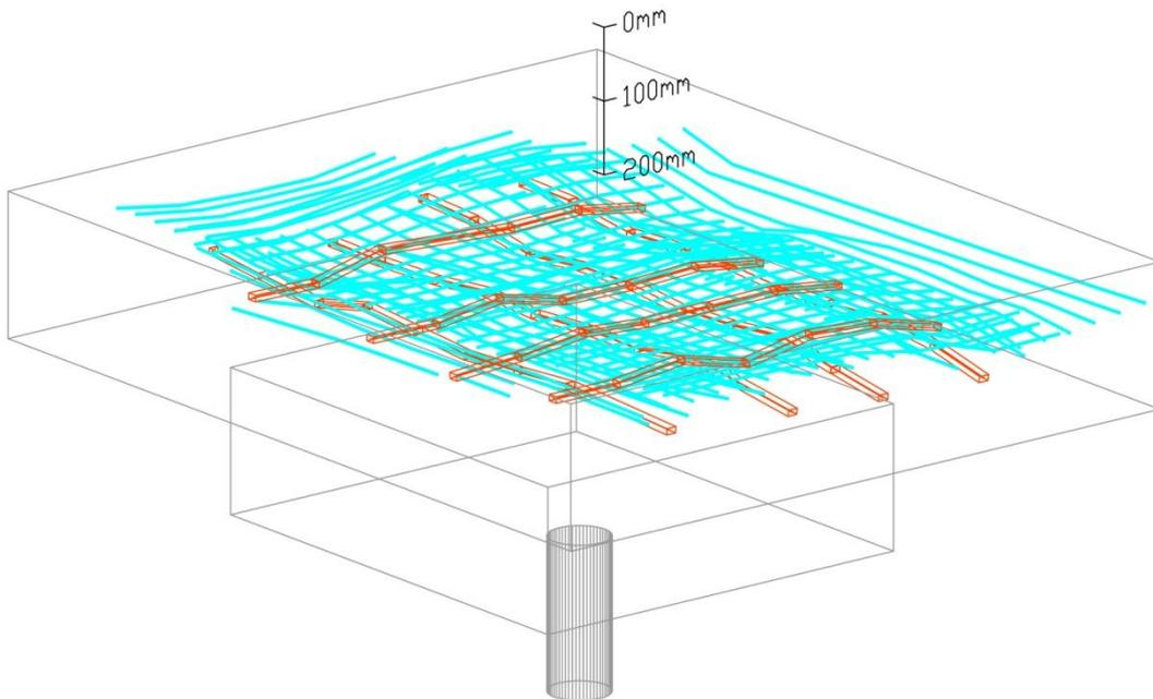
**Figure 6: 3D view of PT duct layout and reinforcement detail**
