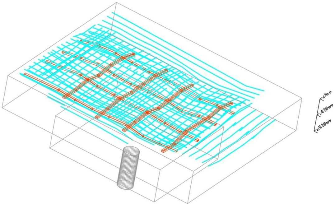
**Figure 5: 3D view from downward perspective view showing PT duct layout and reinforcement detail**
