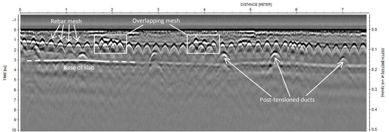
**Figure 3: GPR profile showing features visible within slab**
