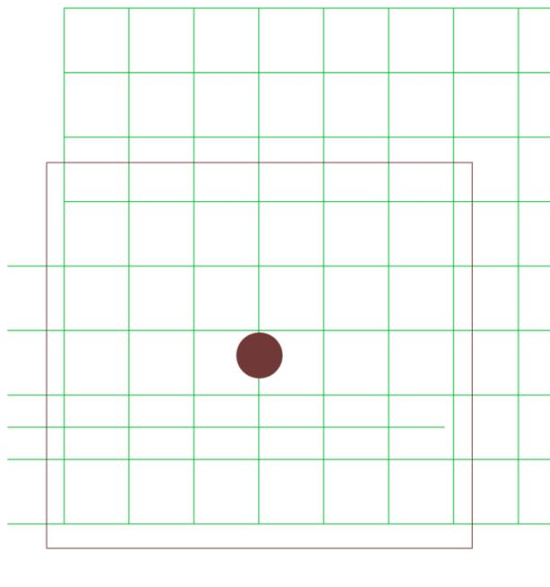
**Figure 2: View of the topside of the slab showing GPR transects (green lines), results of which have been used to create the 3D drawing, line spacing is 0.5m.**
