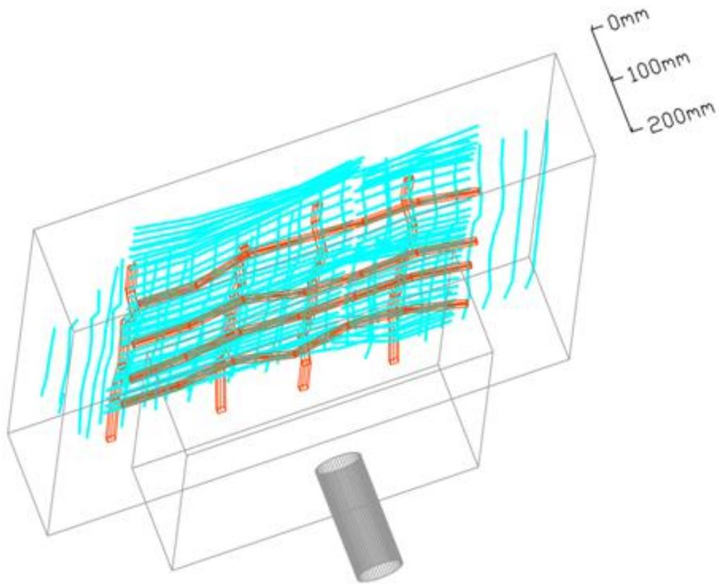
**Figure 7: 3D view from upward perspective view, showing PT duct layout and reinforcement detail**
