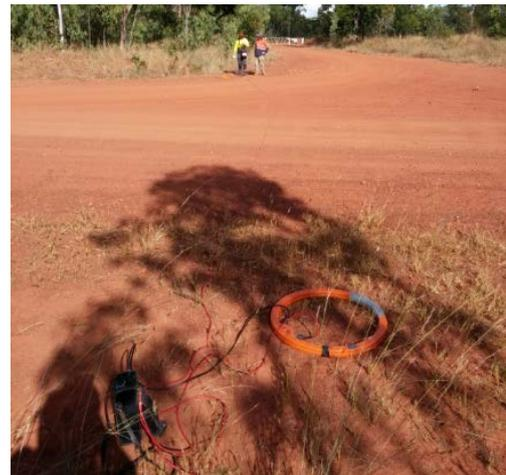
The EM34-3 is a proven tool for groundwater prospecting. Paleochannels are often associated with an increase or decrease in ground conductivity relative to surrounding material.
